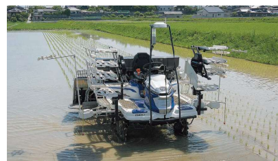
Manned monitoring-based robot rice transplanters which promote high expectations for further laborsaving
